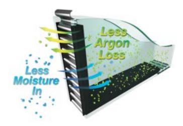
They also need to last a long time under adverse conditions inside your window frame. Duraseal is designed to seal your window better and longer, while increasing energy savings compared to other types of spacers.
